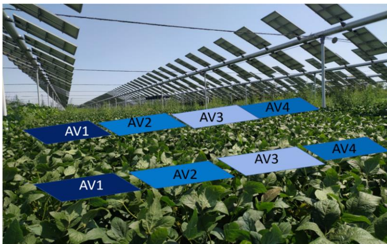
Figure 12: Experimental setup of the soybean trial in Monticelli D'Ongina (2021). Different colours represent the different shade depth (SD) levels, and the four SD levels are indicated as follows: AV1 = 27%, AV2 = 16%, AV3 = 9%, and AV4 = 18% (Potenza et al., 2022)
